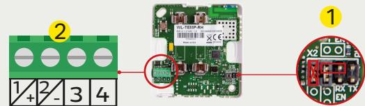
2. Connect the transmitter measurement to terminal strips 3 and 4 (power source's ground **1**) **2**
