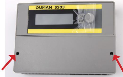
Open the front cover screws and remove the front cover.
