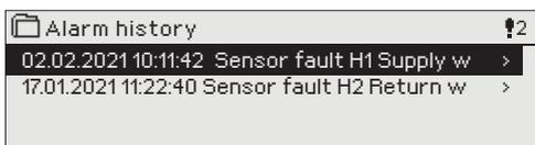
The reason, source and inactivation time (02.02.2021 10:11:42) is shown for every alarm in alarm history. The last 10 alarms can be seen in inactive alarms.
