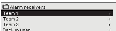
A GSM modem can be connected to the S203 for alarm sending a text message to the alarm team. The alarms are sent to correct team according to alarm routing schedule. When alarm is activated, the controller sends alarm messages automatically to phone numbers defined in team. If the alarm isn't acknowledged within 5 minutes, the alarm message will be re-sent to same recipients and also to backup number. The S203 send max. 100 within one day.
