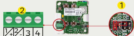
1. Remove the battery-side short-circuit (jumper) and turn the other short-circuit from upright to two middle pins in horizontal position on sensor circuit board.
