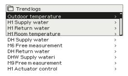
H21 controller automatically logs trend from the measurements. Select the measurement which log you want to view. The trend log will be shown in the controller's display. It's also possible to change the logging interval. By default, the trend log sampling interval for outdoor temperature is 600 s, for DHW Supply water 10 s and for other measurements 60 s.
