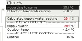
When system works optimally, the supply water temperature is very close to the calculated supply water temperature setting value. The circuit specific info view shows the temperature measu rements and the states of the actuators of the particular control circuit. (moreinformation p.8).
