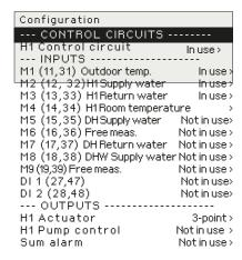
In Configuration menu the heating circuits and the inputs and outputs are configured and taken in use. The service code is needed for the access to the Configration menu.
