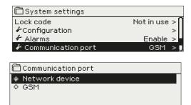
A GSM-modem or network device (M-LINK adapter) can be connected to H21's communication port. M-LINK provides Modbus TCP/IP interface to H21.
