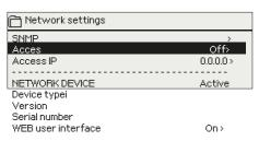
M-LINK supports Ouman Access-service which gives you a secure remote connection to the H21-device. With this setting you can activate the ACCESS-service in order to be able to use it.
