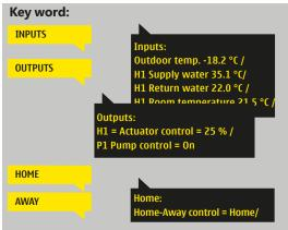
If a GSM is connected to the controller, you can read measurement information form a mobile phone. (If you have a device ID, write the device ID in front of the key word, e.g., TC01 Inputs)
