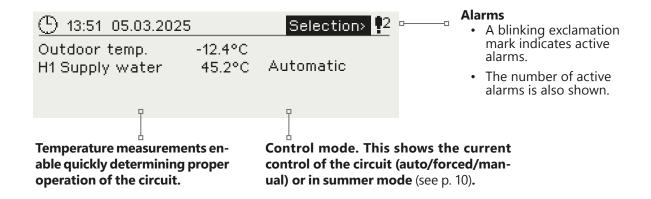
Acknowledging alarms: Press OK and the alarm sound will stop. If the reason for the alarm has not been corrected, the exclamation mark in the top right
