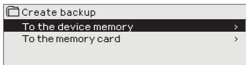
Backup is done in System settings by pressing the OK-button down for an extended period of time (Backup-menu appears to System settings).
