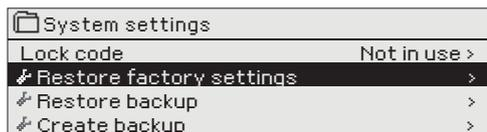
When you return the factory settings, the controller takes into use those control circuits, which were in use before factory reset. The restoring factory settings is done in System settings by pressing the OK-button down for an extended period of time (Backup-menu appears to System settings).
