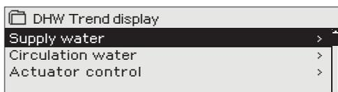
You can read the real-time trends of the temperatures of supply water and circulation water. Also the real-time trend of actuator control in domestic hot water circuit can be read. The sampling interval is 1 s.
